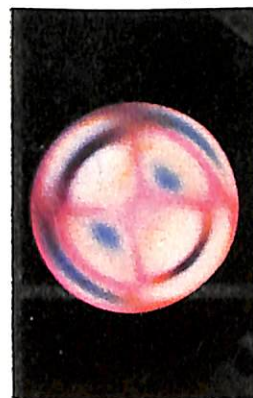
(1) Uniaxial interference figures with the polarizing microscope. (a) Quartz. (b) Calcite. (2) Uniaxial interference figure with gypsum plate (quartz). (Photomicrographs courtesy of ERNST LEITZ GMBH, WETZLAR).
